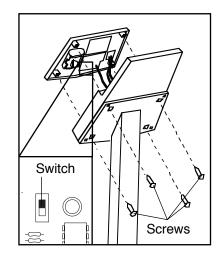
console. Slide the switch up or down to change the unit of measurement. Reattach the console with the four screws; **be careful not to pinch any of the wires.**
